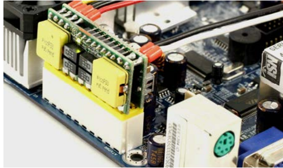
Fig 1.1 picoPSU-120 plugged into ATX connector.
